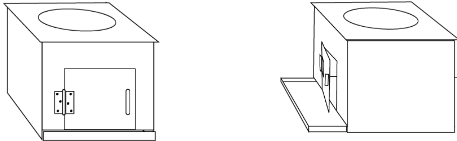
square stove with detachable tray and inner metal lining.
